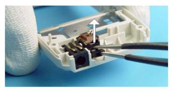
16. To remove the DC jack, place tweezers between the spring contacts and under the jack. You need to use additional force to pull the jack upwards.
