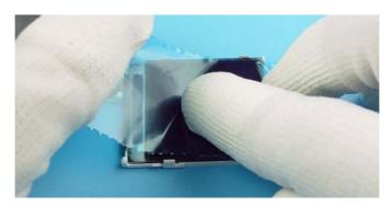
9. Remove the earpiece. Note the guiding pin when re-assembling.
