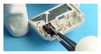
17. Use a flathead screwdriver as a lever to remove the release spring.
