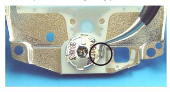
10. The shielding is attached with hooks at its backside. To remove the shielding from the B-cover, first expand the B-cover, then push the shielding upwards.
