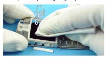
8. Always protect the LCD window with a protection foil to avoid dust and scratches.
