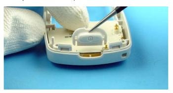
12. Use the SRT-6 to lift up the antenna.
